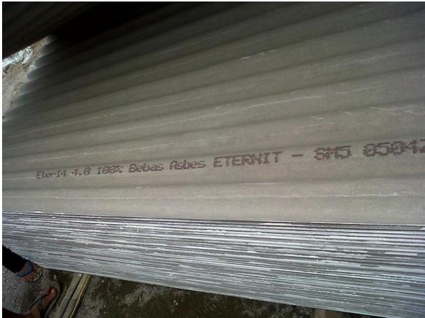
Fiber Cement roof material is 100% asbestos free
